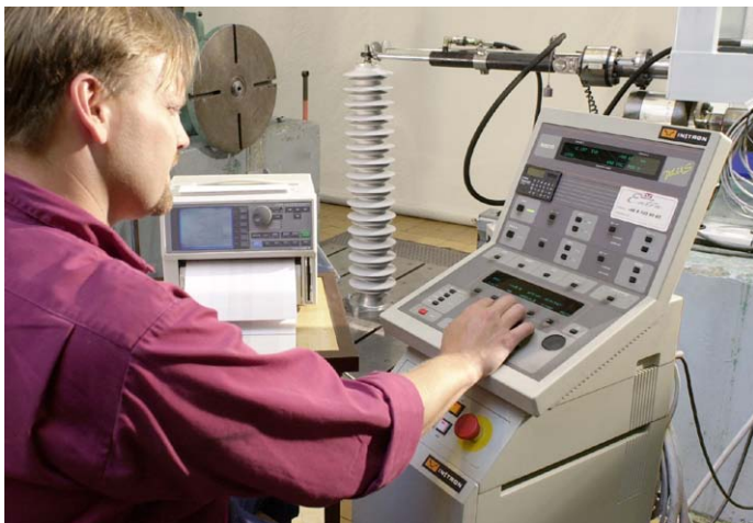
Mechanical test of silicone-housed arrester PEXLIM P.
